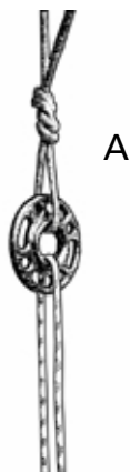
Figure 1. Moving: A single rope passed through the anchor in a moving rope setup.
